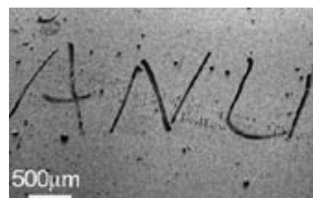
The three letters A, N and U shown here are each composed of millions of carbon nanotubes (pictured above) grown on top of a scratch on a silicon wafer. The nanotubes were grown by researchers in the Department of Electronic Materials Engineering.
