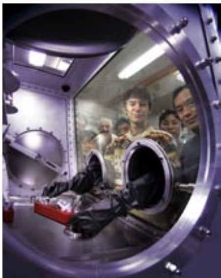
Handling of the ultra-fine powders used to generate nanotubes has to be carried out in a special controlled atmosphere glovebox.
