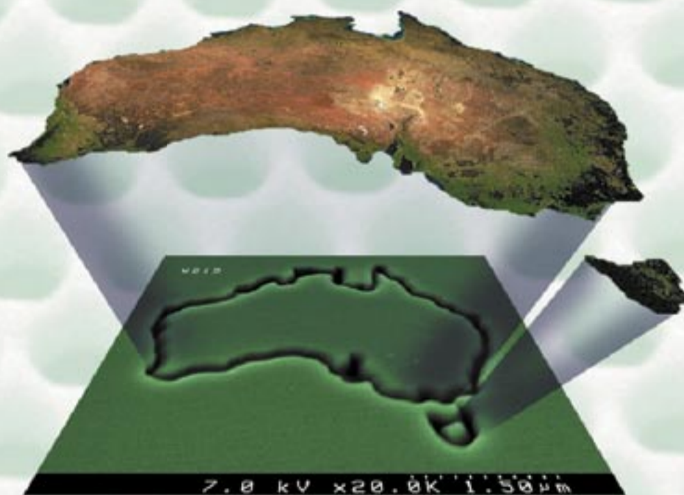
Demonstrating the versatility of the focussed ion beam mill: a map of Australia only few wavelengths of light across, cut into the surface of glass
